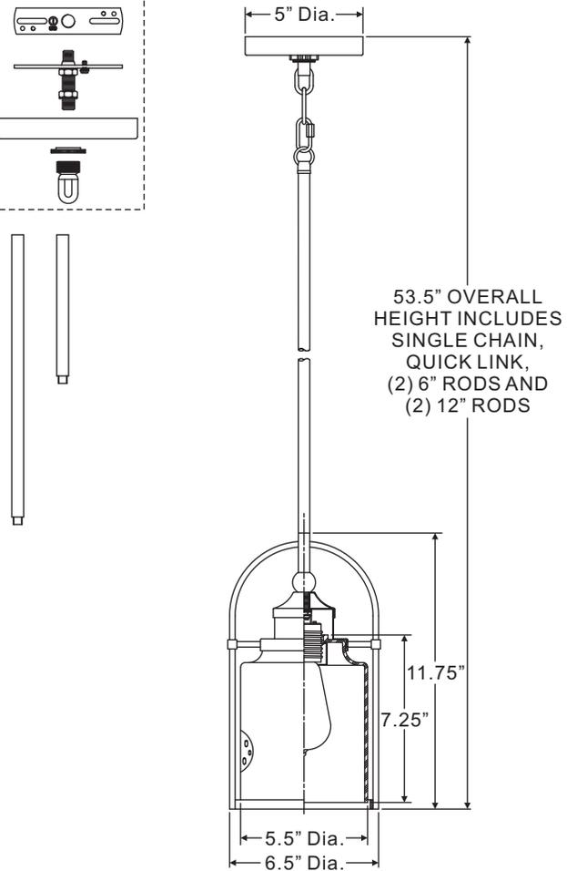
53.5" OVERALL HEIGHT INCLUDES SINGLE CHAIN, QUICK LINK, (2) 6" RODS AND (2) 12" RODS
