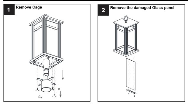
Reverse above steps to reinstall the replacement Glass Panels onto fixture.
