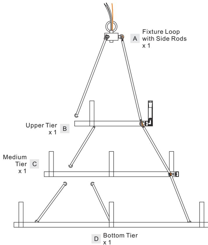
**STEP 1 – Install Fixture Loop with Side Rods, Upper Tier, Medium Tier and Bottom Tier together**
